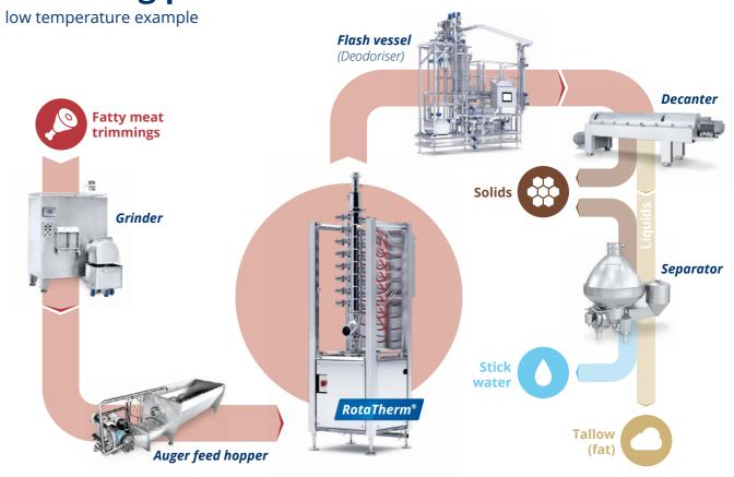
44,000lbs per hour of fatty beef meat trimmings are transported to a grinder, and ground through a hole plate, usually 1/8 to 3/16. This product will generally test about 70% fat.
